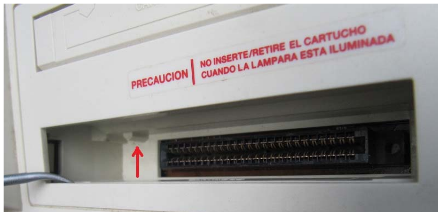
Figure 2. Ridge in the system's cartridge slot (above the red arrow)
