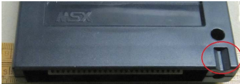
Figure 1. Notch in the back of a cartridge
