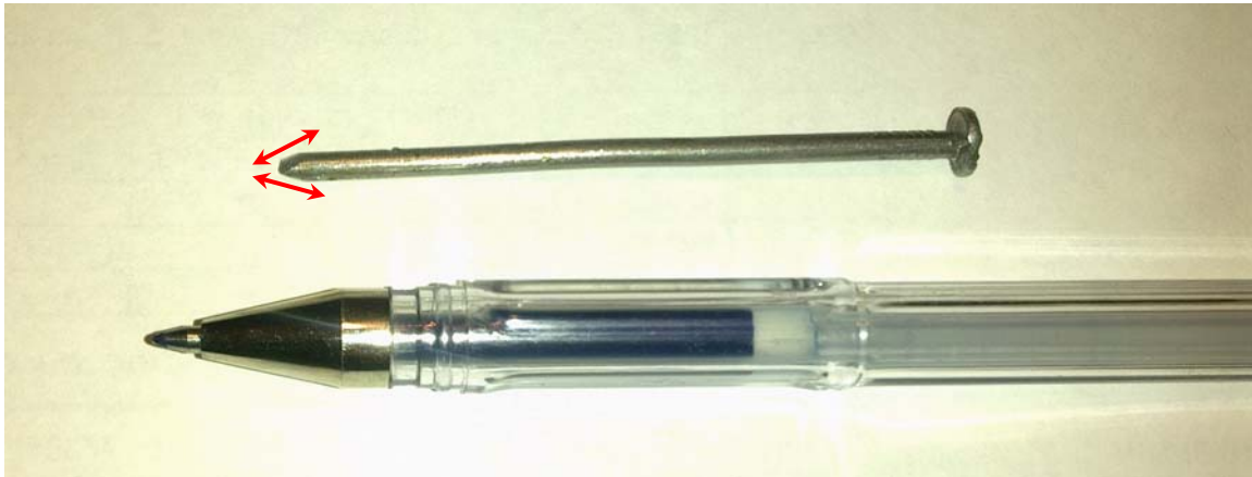
Figure 3. Nail converted to the small screwdriver (at the top)
