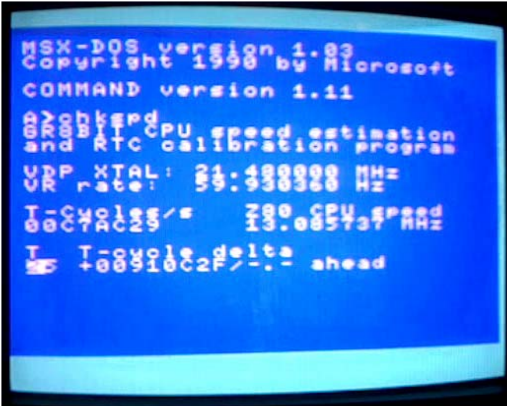
Figure 8. Running CHKSPD on the accelerated GR8BIT: as CHKSPD is not designed for variable speed designs, it displays slightly wrong results. Value of XTAL1 installed is 12MHz, not 13MHz.
