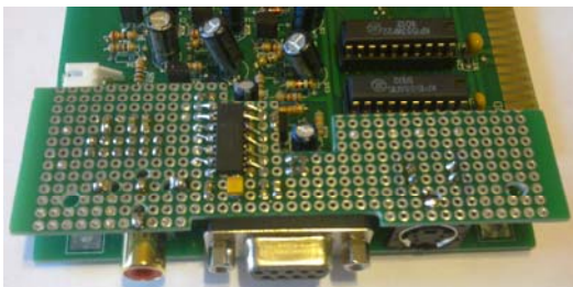
(o) solder components onto outer surface
